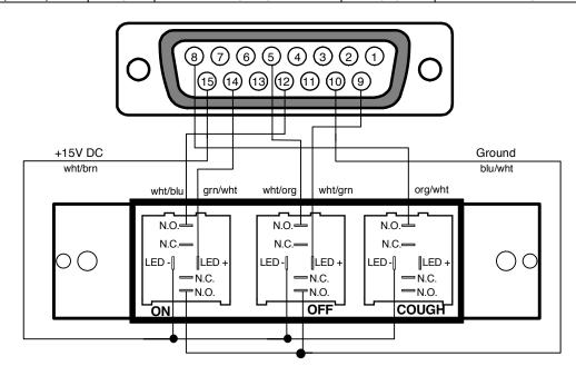
Model SH-3BUT 3 Push Button Plate with 15V LED shown Also available – Model SH-3BUTRC with RJ-45 connector
