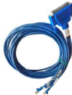
Analog Audio 4-Input Cable Part # LAWO-ANALOGIN DB-37 male (mates with DB-37 female on Lawo chassis) to 4 StudioHub+ RJ-45 males on 6' cable
