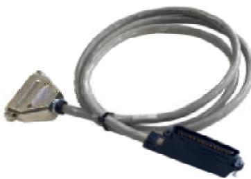
GPIO Break-Out Cable Part # RJ21RCD50M-XXX DB-50 male (mates with DB-50 female on Lawo chassis) to 4 RJ-21 male (mates to RJ-21 female on punch block) (XXX = specify length in feet)
